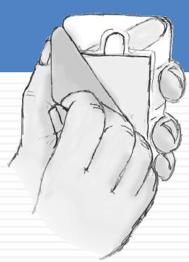
Peel back the package to remove the device. Hold the device with your thumb on the bottom of the plunger and 2 fingers on the nozzle.
